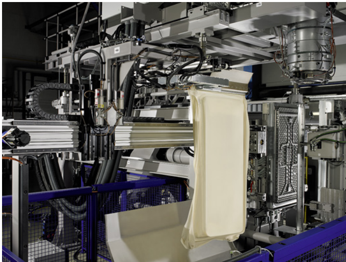
Figure 1.9 Extrusion blow molded flat panel (table top) (Image: Kautex Maschinenbau)
