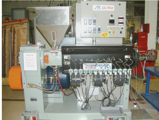
Figure 1.1 Photograph of a highly instrumented 63.5 mm diameter extruder built by American Kuhne
