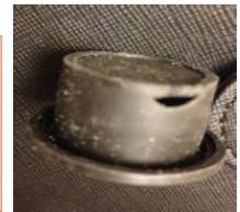
Figure 25.7 Weld lines between two flow fronts can cause air entrapments
