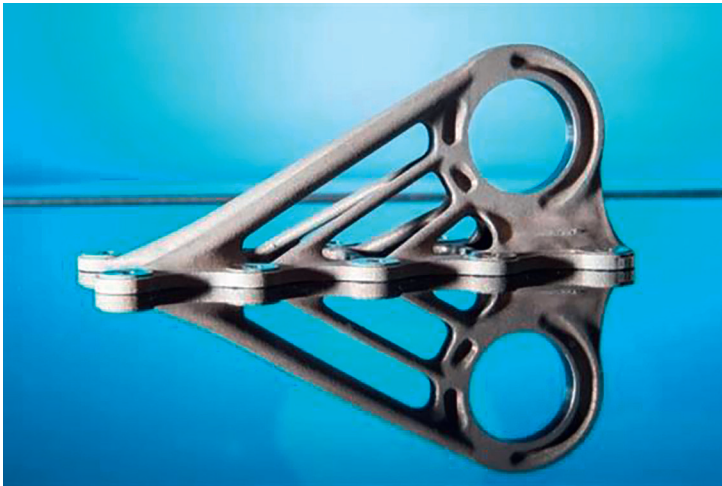
Figure 4.9 3D printed lightweight bracket, for the A350 XWB; SLM, titanium (Source: Airbus)
