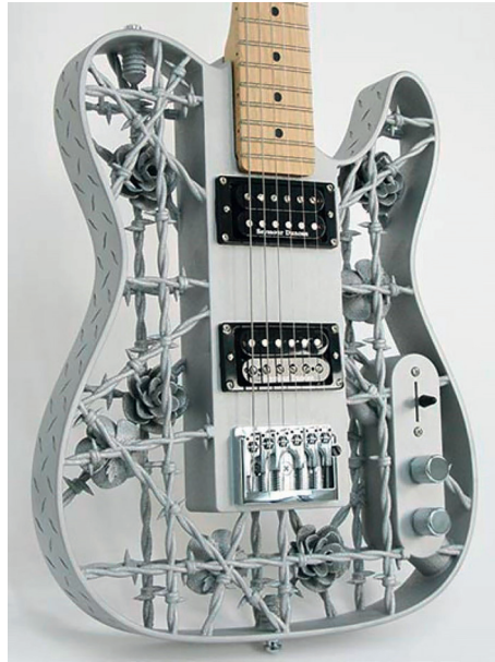
Figure 4.16 3D printed guitar made from aluminum, SLM (Source: Xilloc/Diegel)
