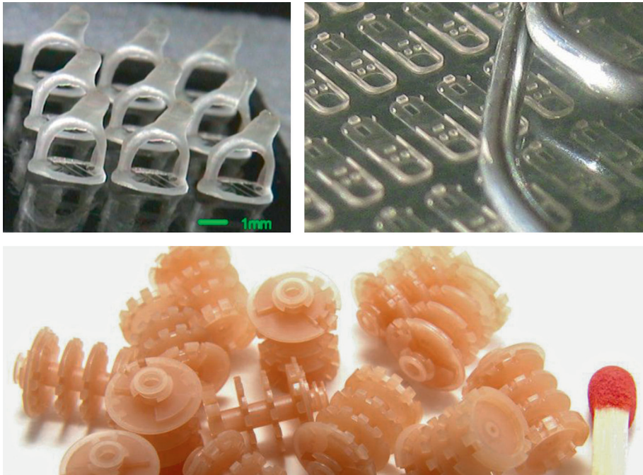
Figure 2.10 Micro stereolithography, parts and MEMS (microelectromechanical systems) (Source: microTEC)
