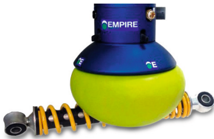
Figure 3.34 Example of Versaball application (source: KurtwoAI 66 )
