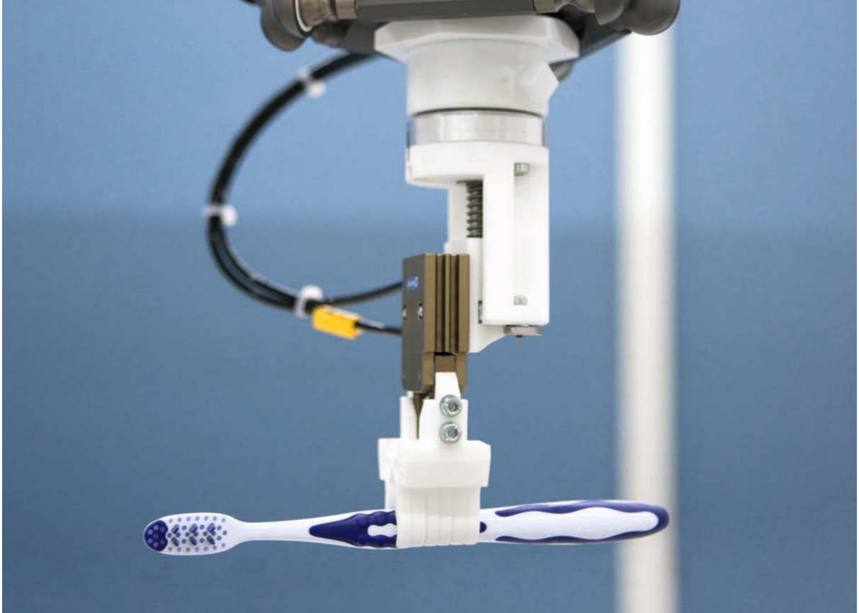
Figure 3.36 Flexible retracting gripper finger for different toothbrush geometries (source: Zahoranskey 81 /robomotion 60 )
