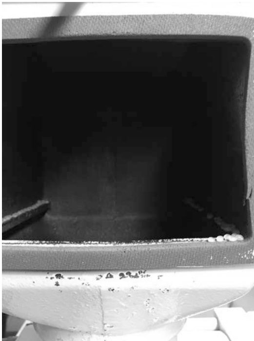
Figure 23.2 Pellets stuck in magnet drawer
