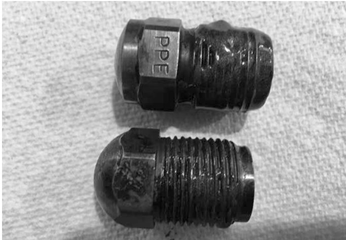
Figure 23.6 Nozzle tip with excess anti-seize (top) and appropriate amount of anti-seize (bottom)
