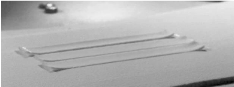
Figure 3.14 Massive curling in the first layers of the part [source: Inspire AG]
