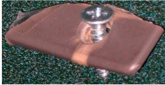
Figure 3.43 White stress cracking marks with flat head screw in a polyethylene part
