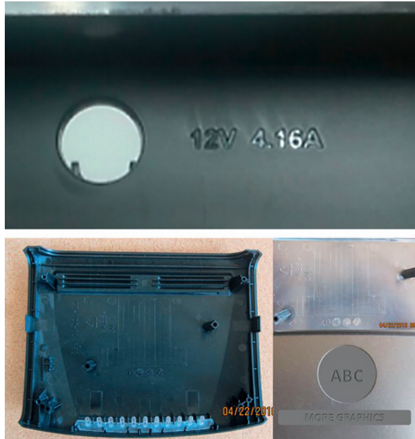
Figure 5.43 Deep graphics causing interruption of flow
