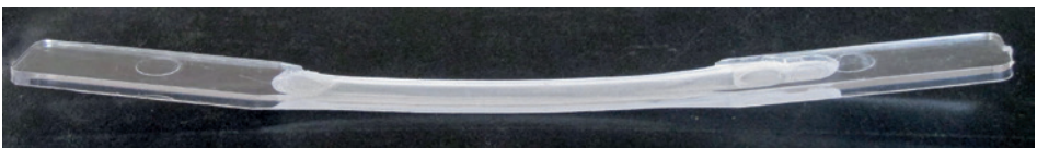
Figure 2.37 Stress relief with machining
