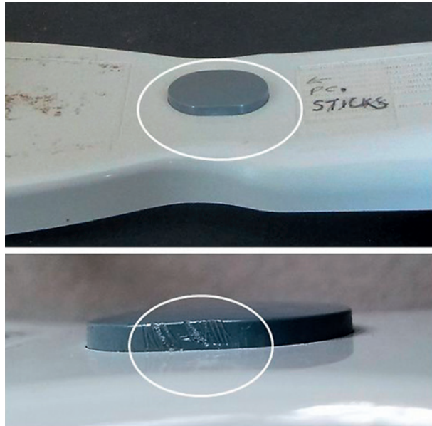
Figure 3.66 Trigger button failure: the circled area shows vertical wear scratches on the button
