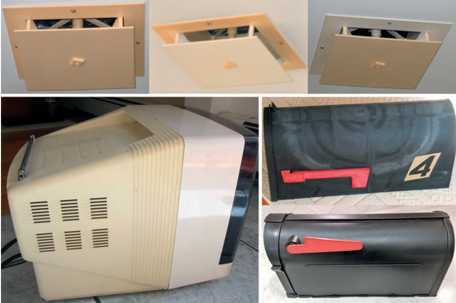
Figure 2.30 Long term yellowing and fading of plastics
