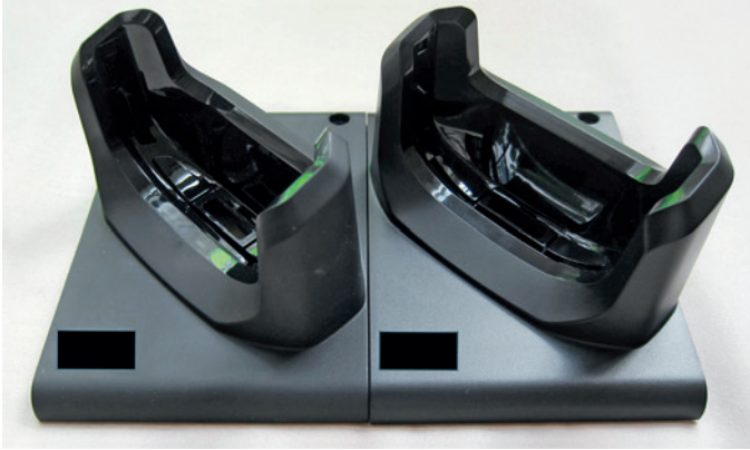
Figure 5.25 The left view shows a part with lower mold temperature and pressure; the right view shows the same part with higher mold temperature and pressure
