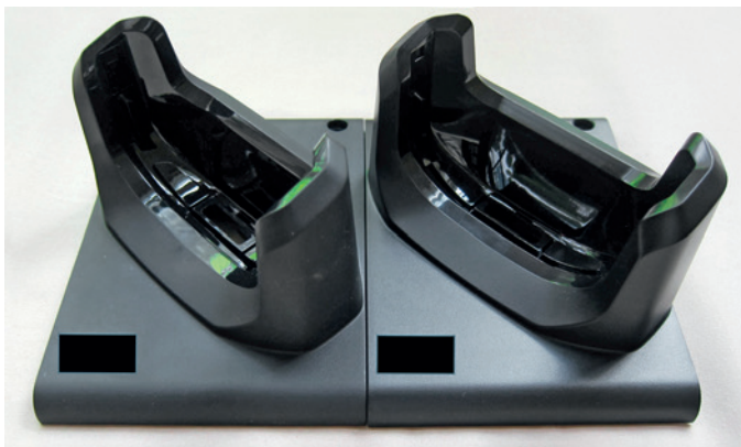
Figure 5.42 Noticeable change in the reproduction and matt level in the textures with the change of mold temperature and/or pack pressure
