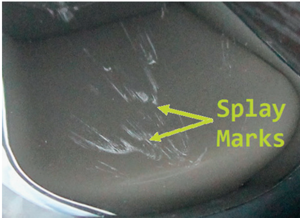
Figure 5.41 Splay due to moisture in the resin [9]
