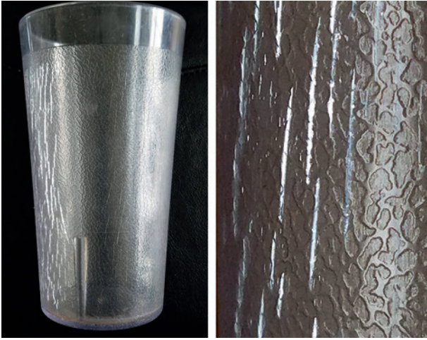
Figure 3.38 Stress crazing in a clear polystyrene tumbler
