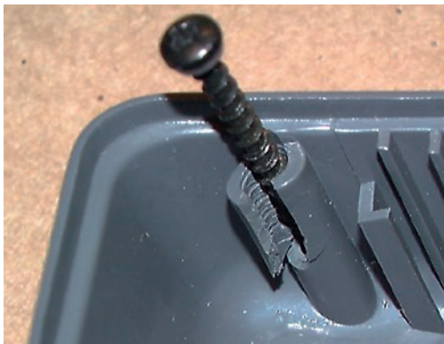
Figure 3.41 Catastrophic failure of PC/ABS part with thread forming screw
