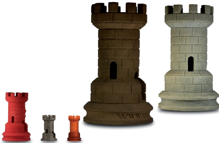
Figure 1.2 Additive manufacturing. Scaled towers of a chess set, based on the same data set but made with different AM machines and from different materials.
