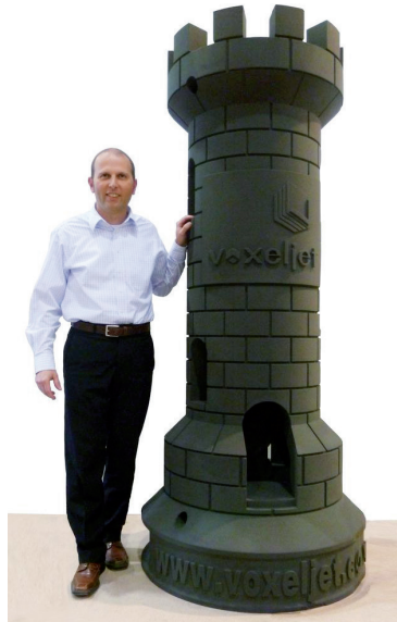
Figure 1.3 Chess tower made from foundry sand, height approx. 2.5 m, powder-binder process (Source: Voxjet)
