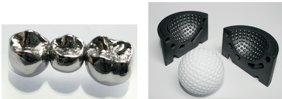
Figure 1.9 Rapid manufacturing: direct manufacturing of a three-element dental bridge (left) (Source: GoetheLab FH Aachen/Sokalla); direct tooling for making golf balls (right) (Source: EOS GmbH)
