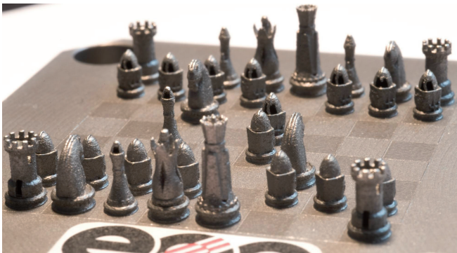
Figure 1.4 Tower made from metal, height approx. 5 mm, micro laser sintering (Source: EOS/3D Micromac)
