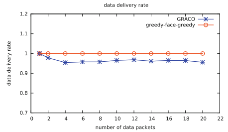
Fig. 8. Delivery rate varying with the number of data packets sent
