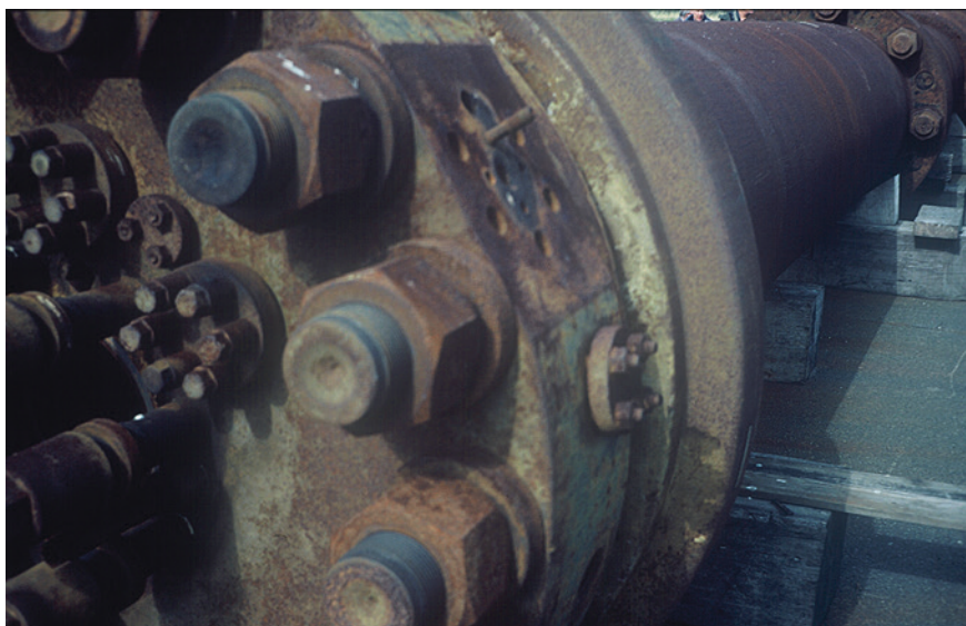
Fig. 2.31 Early BASF Haber-Bosch converter, showing massive bolts and studs required to secure the cover plate. This converter is now preserved at the Wroughton outstation of the Science Museum London
