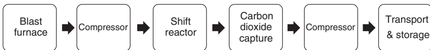
Fig. 2.3 CO 2 capture and storage system process for a conventional blast furnace. Adapted from Gielen (2003)
