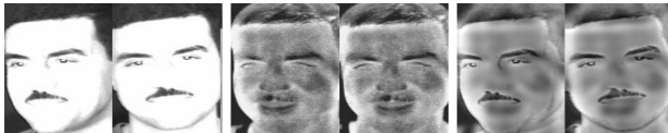
Fig. 1. Visible images (the left two images), infrared images (the middle two images) and the corresponding fused images (the right two images)
