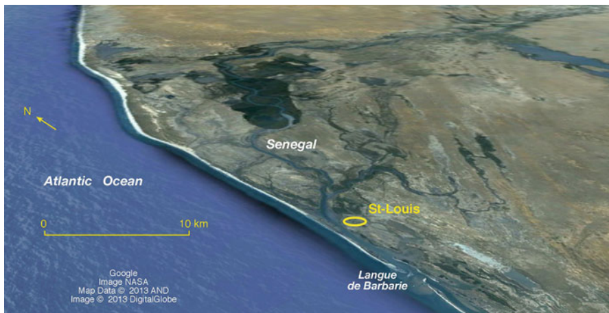
Fig. 2.4 The Senegal River delta, a fine example of a wave-dominated delta characterised by the Languede Barbarie spit and river-mouth system subject to strong north-south longshore drift. This Google image shows a much widened river mouth in 2013 that developed very rapidly from an artificial breach created to prevent river flooding of St. Louis in October 2003. The former natural mouth much further south (sector not shown here) has been sealed by longshore drift
