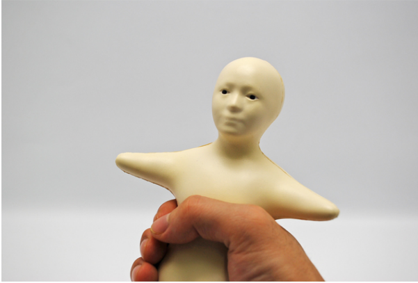
Fig. 1. Cellphone-type tele-operated android: Elfoid. It is important to convey the facial expressions of the speaker to increase communication modality.
