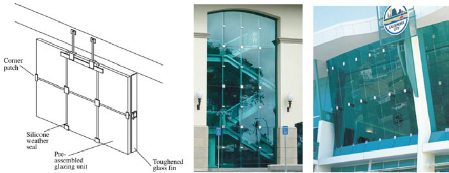
Fig. 2.13 Patch structural glazing
