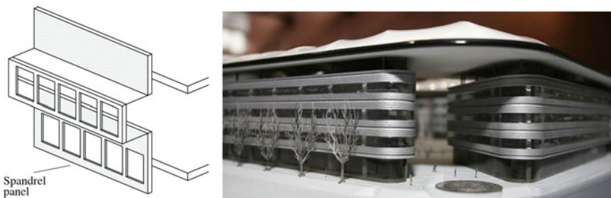
Fig. 2.10 Spandrel ribbon curtain wall systems
