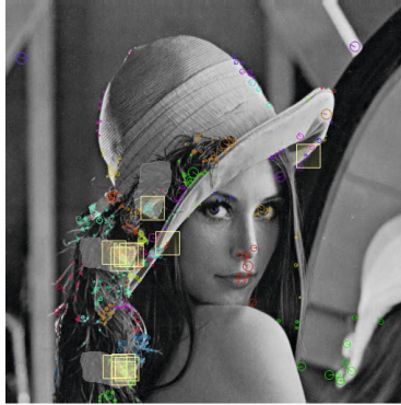
Fig. 2. Detected regions (squares) and SIFT features (circles). The manipulated regions are outlined for convenience only; the input to the algorithm was the image shown in Fig. 1 (center).
