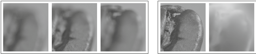
Fig. 5. Coffee bean (provided by the Computer Graphics Group, MPI for Informatics, Saarbrücken, Germany). (a) Left box: 3 out of 22 images of the focal stack of a coffee bean. (b) Right box: Reconstructed sharp image along with the estimated depth ( \alpha = 160 ).
