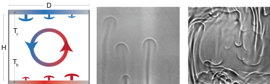
Fig. 2 The image on the left shows a diagram of a Rayleigh-Bénard convection cell. The shadowgraph images from Xi et al. (2004) show the structure of the thermal plumes and the mean wind into which they organize
