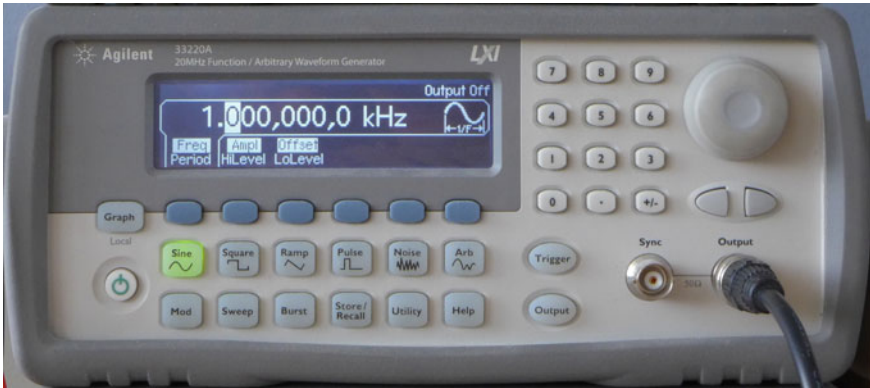
Fig. 2.12 A function generator produces periodic signals within a frequency range from 1 \mu Hz up to several megahertz
