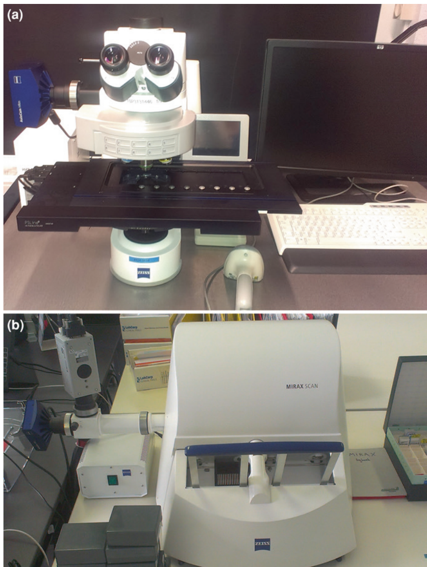
Fig. 2.1 a A Zeiss AxioVision setup with a mounted camera and robotic stage. b A 3DHitech high-volume slide scanner (courtesy of HistoGeneX)
