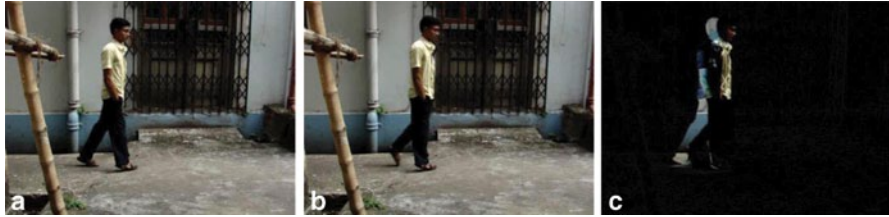
Fig. 2.1 Temporal frame differencing. (a) Present Frame (PF) (b) Previous Frame (Prev) (c) Result=PF-Prev
