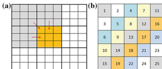
Fig. 2.5 Calculation of cells in the similarity matrix D by using the wavefront approach. Calculation is performed for cells at diagonals, since their values depend on previously calculated cells. Arrows show dependences of particular cells and the direction of value derivation
