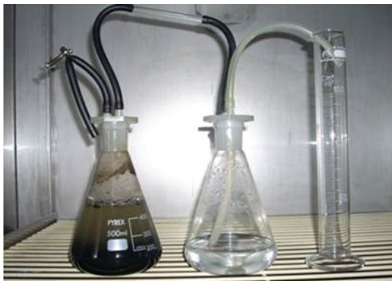
Fig. 2.1 Schematic view of batch test conducted in Erlenmeyer flask Gas production was measured by the water-replacement method
