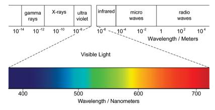
Figure 1.2 Spectrum of electromagnetic radiation.
