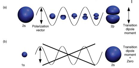
Figure 1.7 (a) The oscillating electric field component of light can induce a transition from an s to a p orbital when it has the correct polarization (direction of oscillating electric field component of light). Please note that here probability densities and not wave functions are visualized. The response of the
