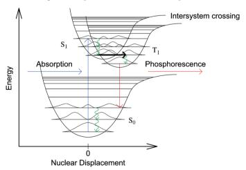
**Figure 1.16** Visualization of triplet-state formation (intersystem crossing) and phosphorescence.
