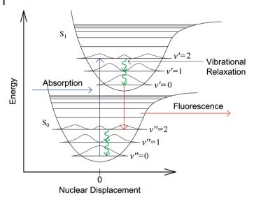
**Figure 1.11** After excitation of a molecule (blue) usually very rapid vibrational relaxation (green) occurs in the excited state. As a consequence, fluorescence (red) normally occurs from the lowest vibrational level of the excited state,  $S_1(v'=0)$ .
