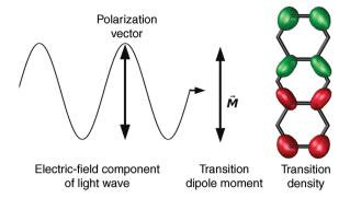
Figure 1.9 Schematic representation of the optimum direction of the oscillating electricfield component of light (polarization vector) in relation to the direction of the transition dipole moment and the corresponding transition density for a  $\varphi_f \leftrightarrow \varphi_h$  transition in
