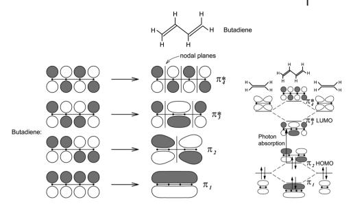
Figure 1.5 Schematic construction of an extended molecular  $\pi$ -orbital system from conjugated atomic p-orbitals. The example corresponds to butadiene. The HOMO and LUMO of butadiene correspond to the  $\pi_2$  and  $\pi_3^*$  orbitals, respectively. The four molecular orbitals  $\pi_1$ ,  $\pi_2$ ,  $\pi_3^*$ ,  $\pi_4^*$  of butadiene can also be
