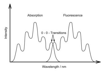
Figure 1.12 Because the potential curves and vibrational wave functions for the electronic ground and excited states of a molecule, are often very similar and symmetric for small v in many cases a mirror symmetry of absorption and fluorescence spectra can be observed.
