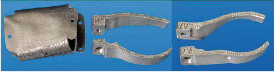
Fig. 2. Implant and cutting templates, manufactured with LaserCUSING®
