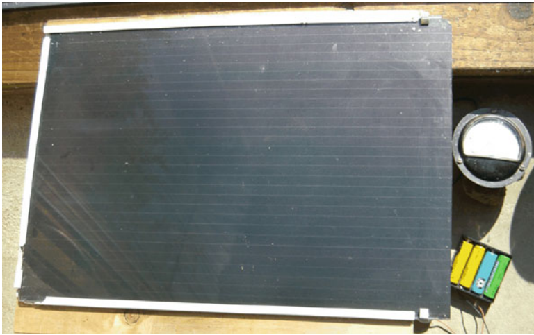
Fig. 2.30 A 14 V solar panel. (In the background are rechargeable “AA”s plus an old ammeter)
