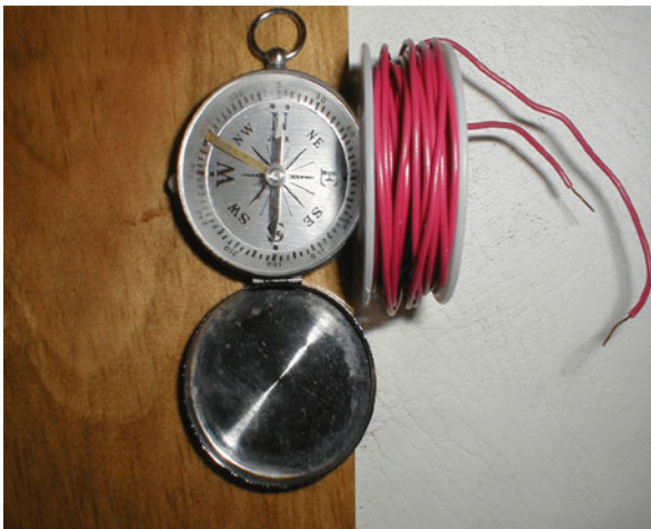
Fig. 2.14 Coil of insulated wire placed as close as possible to compass (it doesn’t matter if it touches the frame of the compass). This is our current meter. Note how we have set it so that the compass originally points north. (Take no notice of the brass marker)
