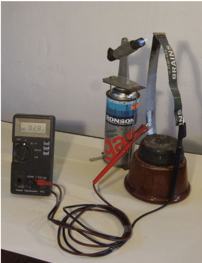
Fig. 2.17 Two dissimilar metal strips, cleaned, joined firmly, and heated (here by a blowtorch). To get even a small reading on the voltmeter one joint must be very hot— so extreme care should be taken . The apparatus could alternatively be set up with the strips approximately horizontal, and then the hot joint could be on a gas or an electric ring
