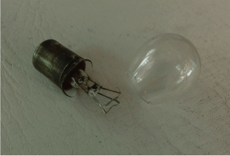
Fig. 2.12 A broken 12 V automobile lamp with two filaments. Without the nitrogen-filled glass bulb the filaments would quickly burn up
