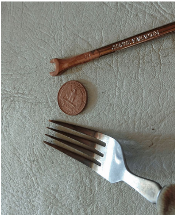
Fig. 2.5 Copper plating of various objects: A chrome–vanadium wrench, a US quarter (originally a silvery color but actually a nickel alloy), and the tines of a fork
