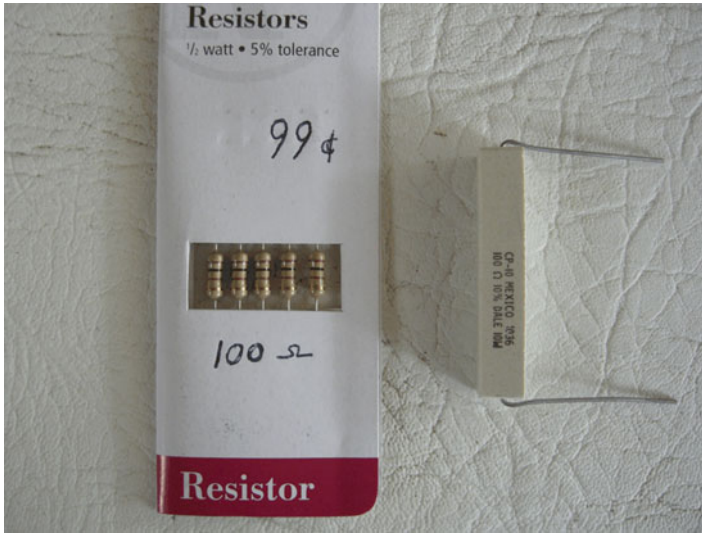
Fig. 2.23 100 Ohm resistors—five low power (“wattage”) and one high wattage
