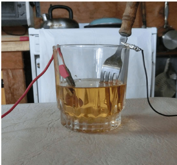
Fig. 2.4 Two electrodes in vinegar. The (+) is a copper penny, and the (–) is the fork or the object to be plated
