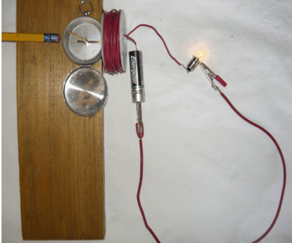
Fig. 2.15 Circuit of Fig. 2.11 modified to include our “ammeter.” After connection the compass needle has swung round strongly (direction shown by pencil direction ). Again brass marker is irrelevant
