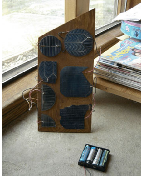
Fig. 2.29 Some “reject” cracked solar cells, glued onto a spare piece of plywood and soldered in series, adding up to \sim 2 V—enough to charge a rechargeable “AA” battery. This little set of broken pV cells has been trickle charging AA camera batteries for many years, one or two at a time (although actually four batteries appear in this photo)
