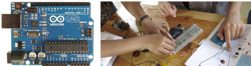
Fig. 2.8 Arduino is an open-source physical computing platform based on a simple microcontroller board and on a system of multimedia programming environment that allows to script and control software for the board. Arduino can be used to develop interactive objects, products and prototypes, since it is able to translate inputs from a variety of switches or sensors into a series of physical outputs controlling lights or motors
