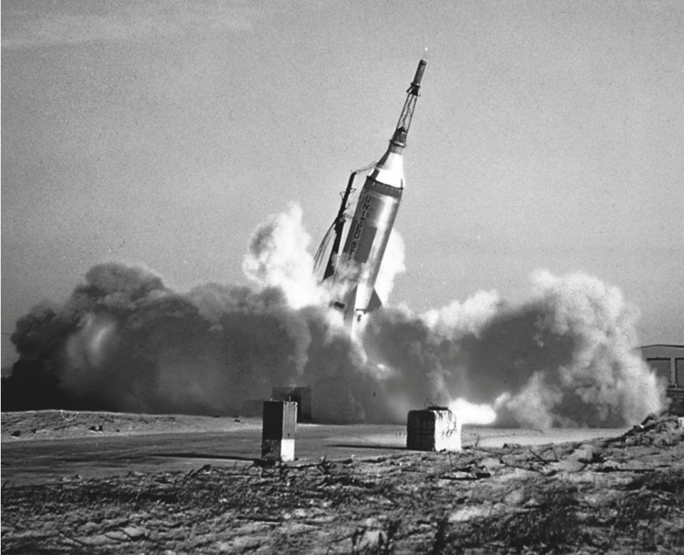
Little Joe LJ-1B, launched on 21 January 1960. The boilerplate capsule used on this primate flight was recovered, and would later be used on the MR-BD flight. (Photo: NASA)
