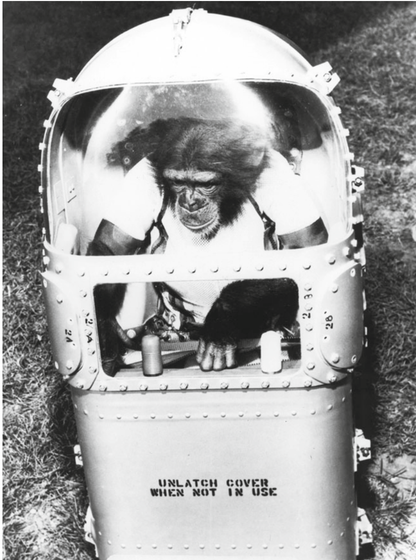
Ham, strapped into his couch and fully enclosed within his space container. Note the psychomotor panel and levers in front of him. (Photo: NASA)
