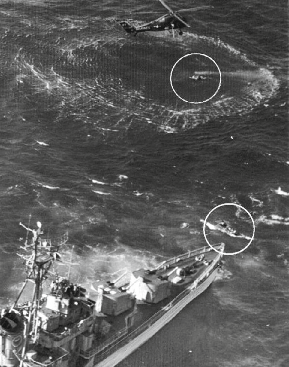
Ham's spacecraft (circled at top) with the recovery helicopter overhead. At bottom (also circled) are two men in a raft near the bow of the USS Ellison . Their task was to right the capsule and help to attach a tow line so that it could be hoisted out of the water. (Photo: U.S. Navy)
