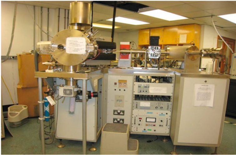
Fig. 2.2 Mass spectrometer at Lamont Doherty earth observatory lab, Columbia university, New York
