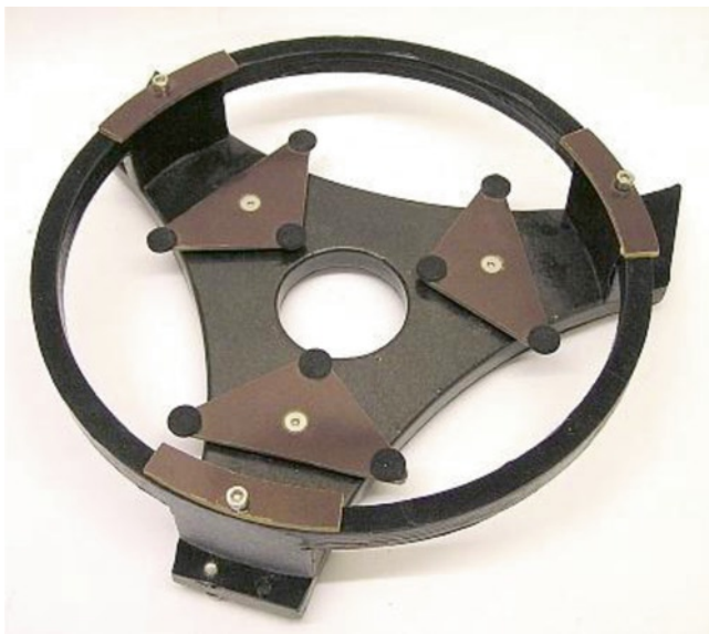
Fig. 2.2. A basic 9-point primary mirror cell (Image credit: John Heath).
