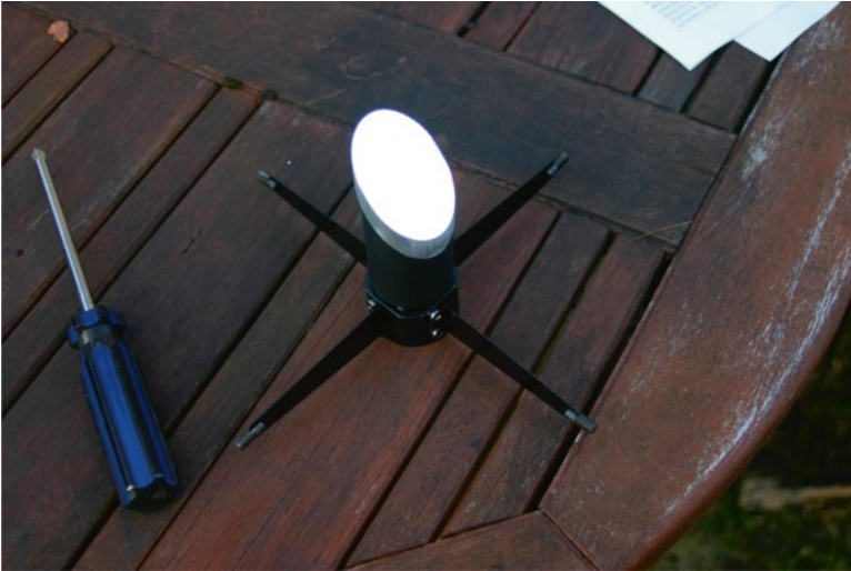
Fig. 2.3. A typical secondary flat mirror attached to spiderlike vanes (Image by the author).
