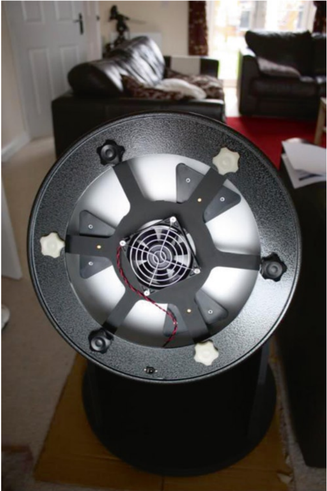
Fig. 2.5. A built-in mirror cooling fan (Image credit: Andy Sheen).
