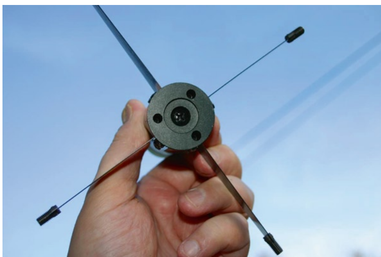
Fig. 2.4. A typical secondary mirror housing for a small Dob (Image by the author).
