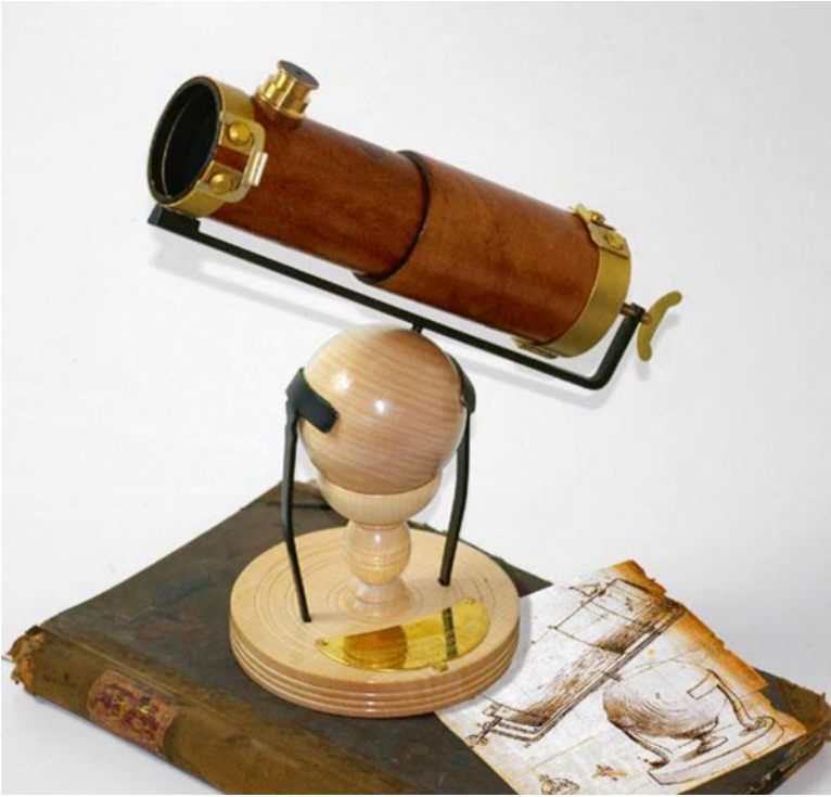
Fig. 2.1. A replica of Newton's reflecting telescope (Image credit: Pulsar Optical).
