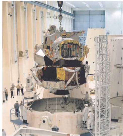
Lunar Module-1, without landing gear, being mated to its adapter. (NASA)
