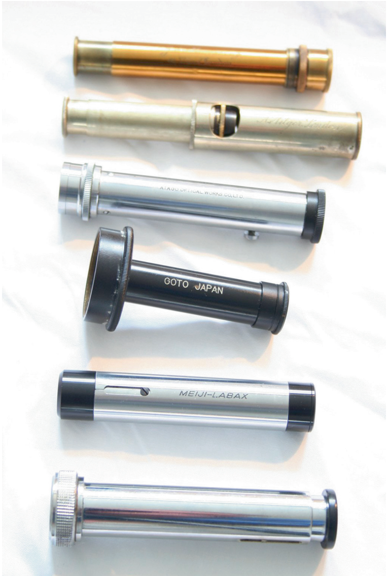
Figure 2.3. Various D-V spectroscopes. From the top: John Browning. (circa 1880), Adam Hilger (circa 1920), LaFayette (1960), GOTO (1970), Meiji-Labax (1980), and Surplus Shed (2004).
