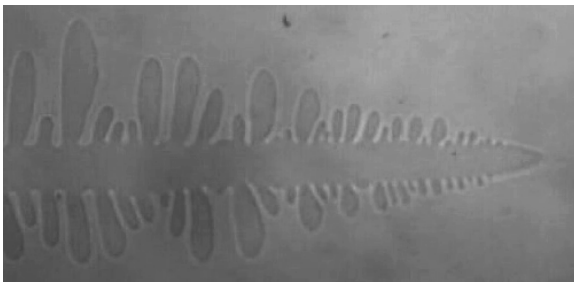
Figure 1.1 A snowflake of succinonitrile, an organic compound that solidified at room temperature. The image shows the characteristic “dendritic” tree-like pattern of the crystal, typical of crystal formation in nearly all
