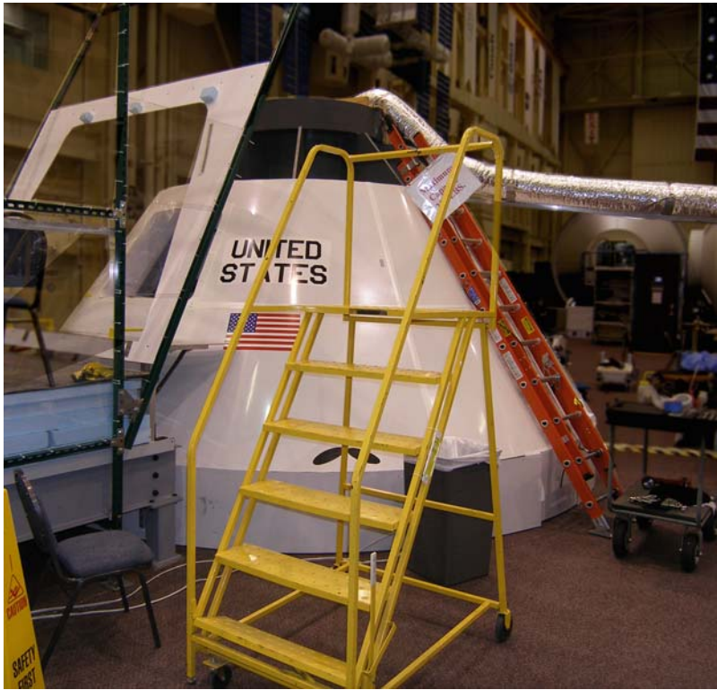
The low-fidelity mockup of Orion has rudimentary couches and is useful for fleshing out the interior space of the CEV. (Photo by the author.)
