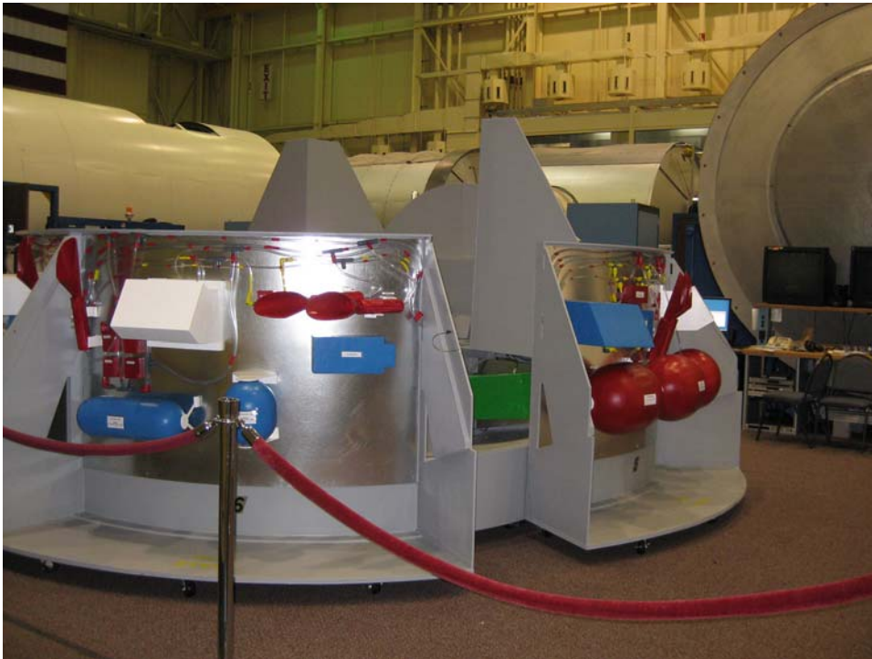
Orion mockup used for arranging systems carried below the flight deck, adjacent to the heat shield. (Photo courtesy of Marianne Dyson.)
