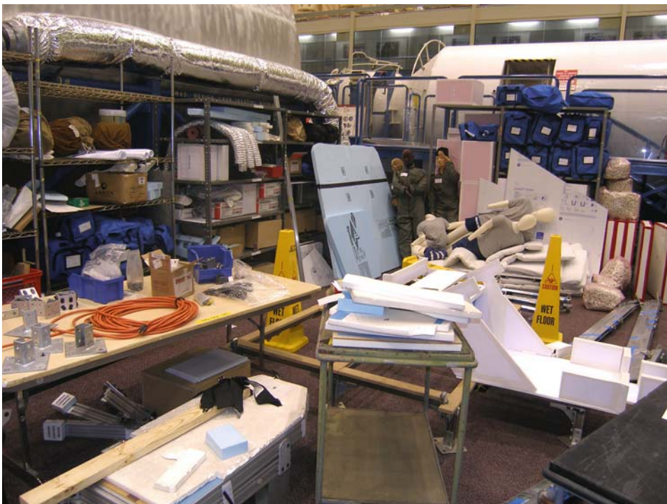
Technicians use cables, hoses, and boxes to size the interior cabin space of Orion. Note manikins for couches and inflatable figures for overhead surfaces used in weightless conditions. (Photo by the author.)
