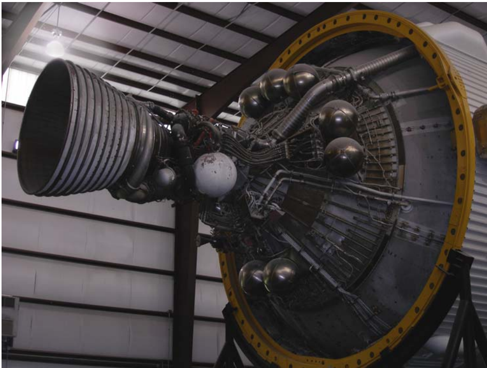
Designers of the Ares family have selected upgraded J-2 engines, whose heritage reaches back to the upper stages of Saturn V, like this one on the Saturn's third stage. (Photo by author.)
