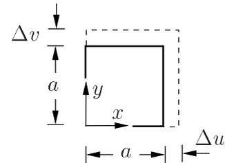
$$\varepsilon_{x1} = \frac{\Delta u_1}{a}, \quad \varepsilon_{y1} = \frac{\Delta v_1}{a}, \quad \varepsilon_{x2} = \frac{\Delta u_2}{a}, \quad \varepsilon_{y2} = \frac{\Delta v_2}{a}$$
