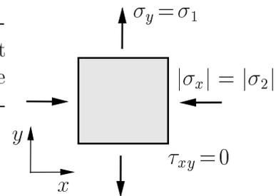
$$\begin{aligned} \sigma_\xi^a &= \frac{\sigma_2 + \sigma_1}{2} + \frac{\sigma_2 - \sigma_1}{2} \cos 2\varphi^a = 22 + 74 \cdot \frac{1}{2} \\ &= \underline{\underline{59 \text{ MPa}}} , \end{aligned}$$
