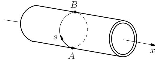
$$\sigma_x^{A,B} = \pm 25 \text{ MPa}, \quad \sigma_s^{A,B} = 50 \text{ MPa}, \quad \tau_{xs}^{A,B} = 50 \text{ MPa}.$$
