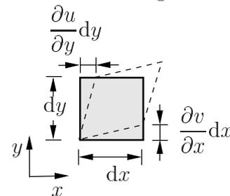
$$\boxed{\gamma_{xy} = \frac{\partial u}{\partial y} + \frac{\partial v}{\partial x}}.$$
