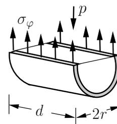
$$\sigma_\varphi \leq \sigma_{zul} \quad \rightsquigarrow \quad p \leq \frac{t}{r} \sigma_{zul} = 1,5 \text{ MPa} \quad \rightsquigarrow \quad \underline{\underline{p_{\max} = 1,5 \text{ MPa}}}.$$
