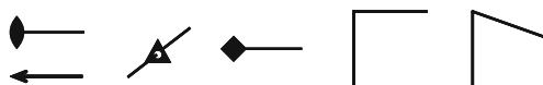
Fig. 2.4 From left to right: horizontal twofold rotation axis ( top ) and its alternative symbol ( bottom ), diagonal threefold inversion axis inclined to the plane of the projection, horizontal fourfold rotation axis, horizontal, and diagonal mirror planes. Horizontal or vertical lines are commonly used to indicate axes located in the plane of the projection, and diagonal lines are used to indicate axes, which form an angle other than the right angle or zero with the plane of the projection.
