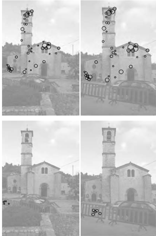
Fig. 11.13 Two different views of Valbonne church. There are two groups, corresponding to two different parts of the scene with different depths. In the first group, the largest meaningfulness is 30.8, in the second group, 2.7 because the resolution is lower in this part
