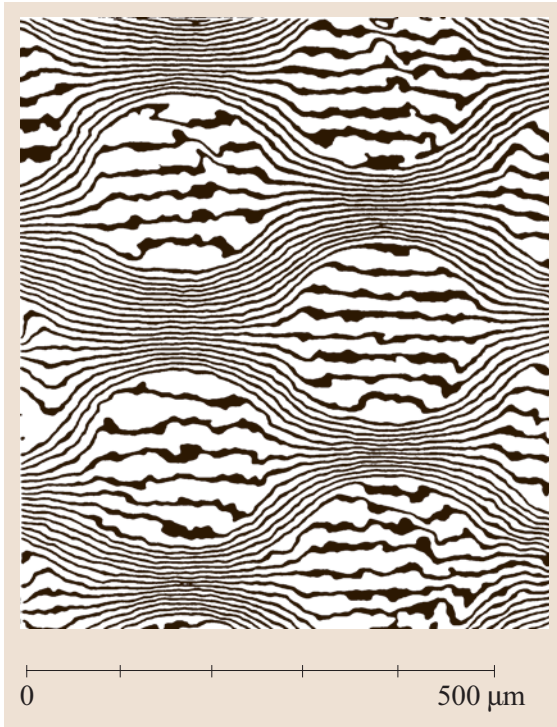
Fig. 1.18 Boron/aluminium composite subjected to a change of temperature of 110 °C. Microscopic moiré interferometry was used with f = 4800 lines/mm and \beta = 6 ; 35 nm/contour
