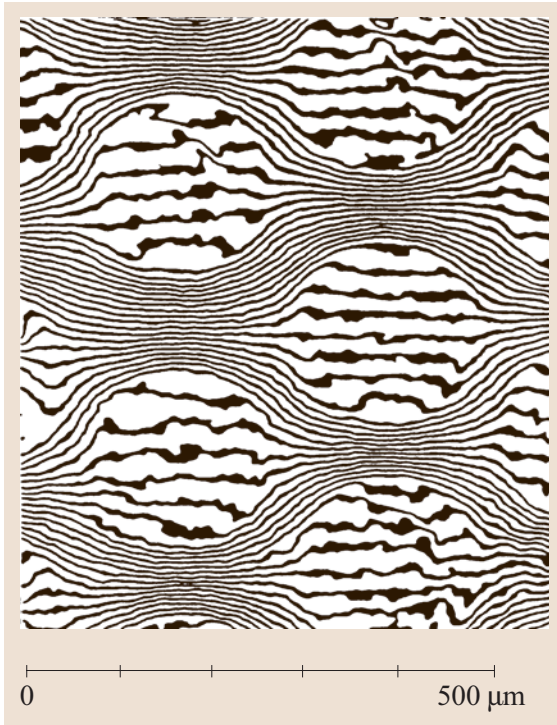
Fig. 1.18 Boron/aluminium composite subjected to a change of temperature of 110^{\circ}\text{C} . Microscopic moiré interferometry was used with f = 4800 lines/mm and \beta = 6 ; 35 nm/contour
