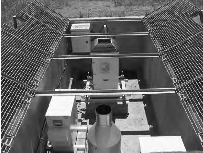
Fig. 4. View of inside of pit with Geonor in foreground and 2dvd in background
