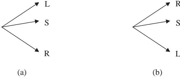
Fig. 2.12. Lax shock condition for traffic flow problem: (a) not a shock, (b) shock
