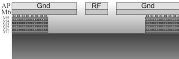
Fig. 2.40 Coplanar transmission line in a 65nm CMOS digital BEOL (6 Metal layers) (© IEEE 2007).
