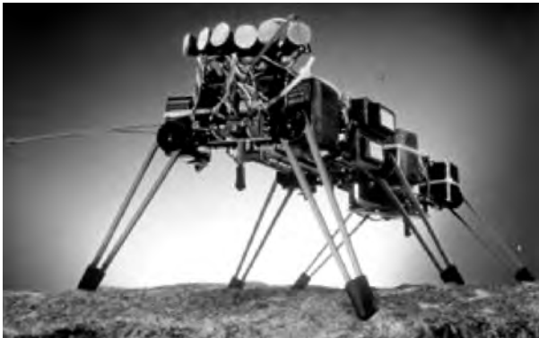
Fig. 1.3. The six-legged walking machine Ghengis . It consists of pitch and roll inclinometers, two collision-sensitive antennas, six forward-looking passive pyroelectric infrared sensors and crude force measurement from the servo loop of each motor. (Photograph courtesy of R.A. Brooks)
