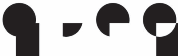
Figure 2.9 Union, intersection, difference and symmetric difference of a circle and a rectangle
