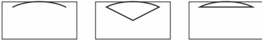
Figure 2.12 An arc of an ellipse, a segment and an arc with its corresponding chord
