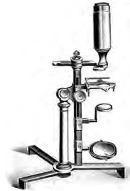
FIGURE 5. W. and S. Jones' 'Most improved' microscope characterises the brass and glass instrument of the late eighteenth century. It was produced in 1790 and influenced designs that were prevalent in the early nineteenth century
