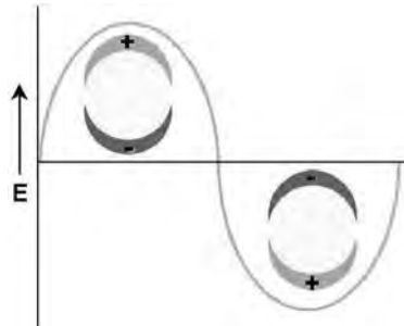
Fig. 1.15. A schematic illustration of the excitation of the dipole surface plasmon oscillation by the electric field component of the light wave. The dipolar oscillation of the electrons has the same frequency as that of the incoming light wave
