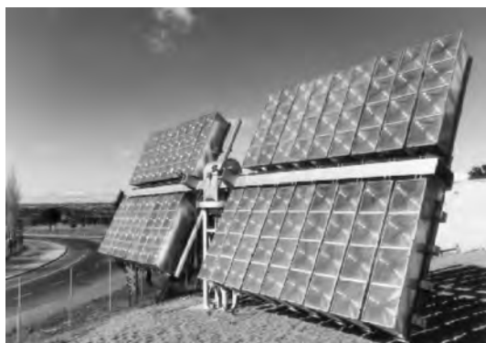
Fig. 1.3. The 1-kWp Ramon Areces Array was developed at ‘Universidad Politécnica de Madrid’, Spain, in 1980. It followed the Sandia Labs concept, but all components were locally made. Curiously, the Fresnel lenses were made of a thin film of silicone stuck on glass, an idea that has recently been taken up again and might be of interest in the future
