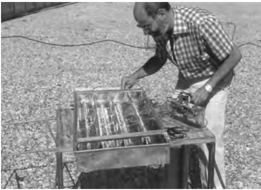
Fig. 1.6. Checking the bifacial cells of a 4.5\times fully static concentrator prototype before filling the module with transparent dielectric (Madrid 1986)
