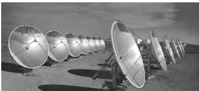
Fig. 1.14. Field of PV parabolic dishes manufactured by Solar Systems in White Cliffs, NSW (Australia). Each dish focuses the light on a compact actively cooled receiver, whose surface is a parquet of BPC cells. Each disk is rated 25 kW p nominal
