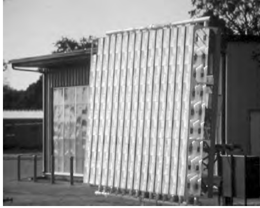
Fig. 1.2. The SANDIA-II array, the first modern PV concentrator made at Sandia National Laboratories, Albuquerque, New Mexico, in 1977. It consist of 5-cm-diameter Si cells operating on two axes under cast acrylic Fresnel lenses at 32 suns, with passive cooling
