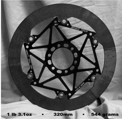
**Figure 1.14** Ceramic matrix composite (CMC) for application as motor-cycle brakes. The CMC is produced from a carbon fiber fabric infiltrated by a SiC forming a pre-ceramic polymer. After the polymer infiltration process (PIP), the device is transformed into a  $C_f/SiC_m$  composite by high-temperature annealing. The Starblade™ brake disc promises an improved brake performance, together with an enhanced lifetime. (Source: Starfire Systems, Inc.)
