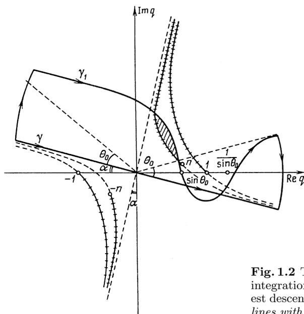
**Fig. 1.2** Transformation of an initial integration path to the path of steepest descent  $\gamma_1$ . The cuts are shown by lines with transverse strokes
